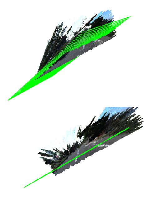
The green point is the 3D point cloud of road that we calculate. We can see that it in the bottom of the image and fit the road plane well.
